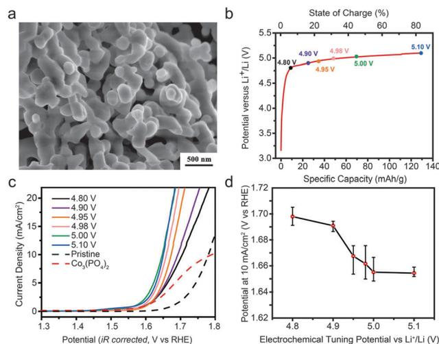
Fig. 2 (a) SEM image of the submicron LCoP particles. (b) A typical charging curve of LCoP. (c) LSV polarization curves (*i*R corrected, vs. reversible hydrogen electrode, RHE) of LCoP charged to different potentials, pristine LCoP and Co<sub>3</sub>(PO<sub>4</sub>)<sub>2</sub> particles in 0.1 M KOH (loading = 0.5 mg cm<sup>-2</sup>). (d) Plots of the electrochemical tuning potentials of LCoP versus the required OER potentials to reach 10 mA cm<sup>-2</sup> current density.
