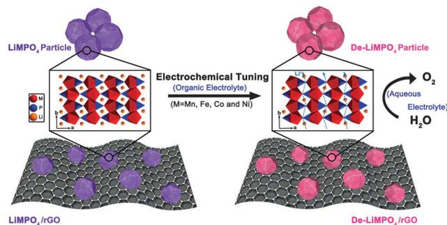
Fig. 1 Schematic illustration of the electrochemical tuning process.
