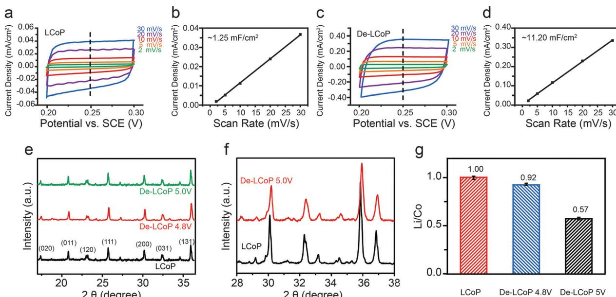
Fig. 4 (a, c) EDLC curves of LCoP and De-LCoP 5.0 V respectively (a with different scan rates; (b, d) plots of current densities at 0.25 V versus scan rates of LCoP and De-LCoP 5.0 V respectively. (e) Powder XRD patterns of LCoP, LCoP 4.8 V and LCoP 5.0 V. (f) Localized XRD patterns of LCoP and LCoP 5.0 V with  $2\theta$  ranging from 28–38°. (g) Li/Co atomic ratio of LCoP, LCoP 4.8 V and LCoP 5.0 V obtained by ICP-MS.
